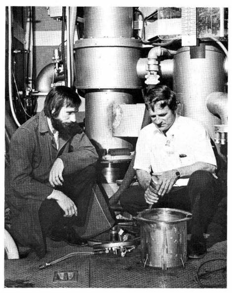
EXAMINING an ingot that has been remelted in the copper chamber behind them are Lee Bertram (2646) and Frank Zanner (5836). Their work on the arc melting process is yielding valuable data that will help manufacturers make alloys with greater homogeneity.
